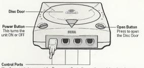
Use these ports to connect the Dreamcast Controller or other peripheral equipment. From left to right are Control Port A, Control Port B, Control Port C, and Control Port D. Use each port to connect controllers for players 1 to 4 respectively. This game is a one player game. Before turning the Sega Dreamcast power ON, connect the controller or other peripheral equipment into the control ports of the Sega Dreamcast.
